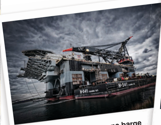
High capacity crane barge
