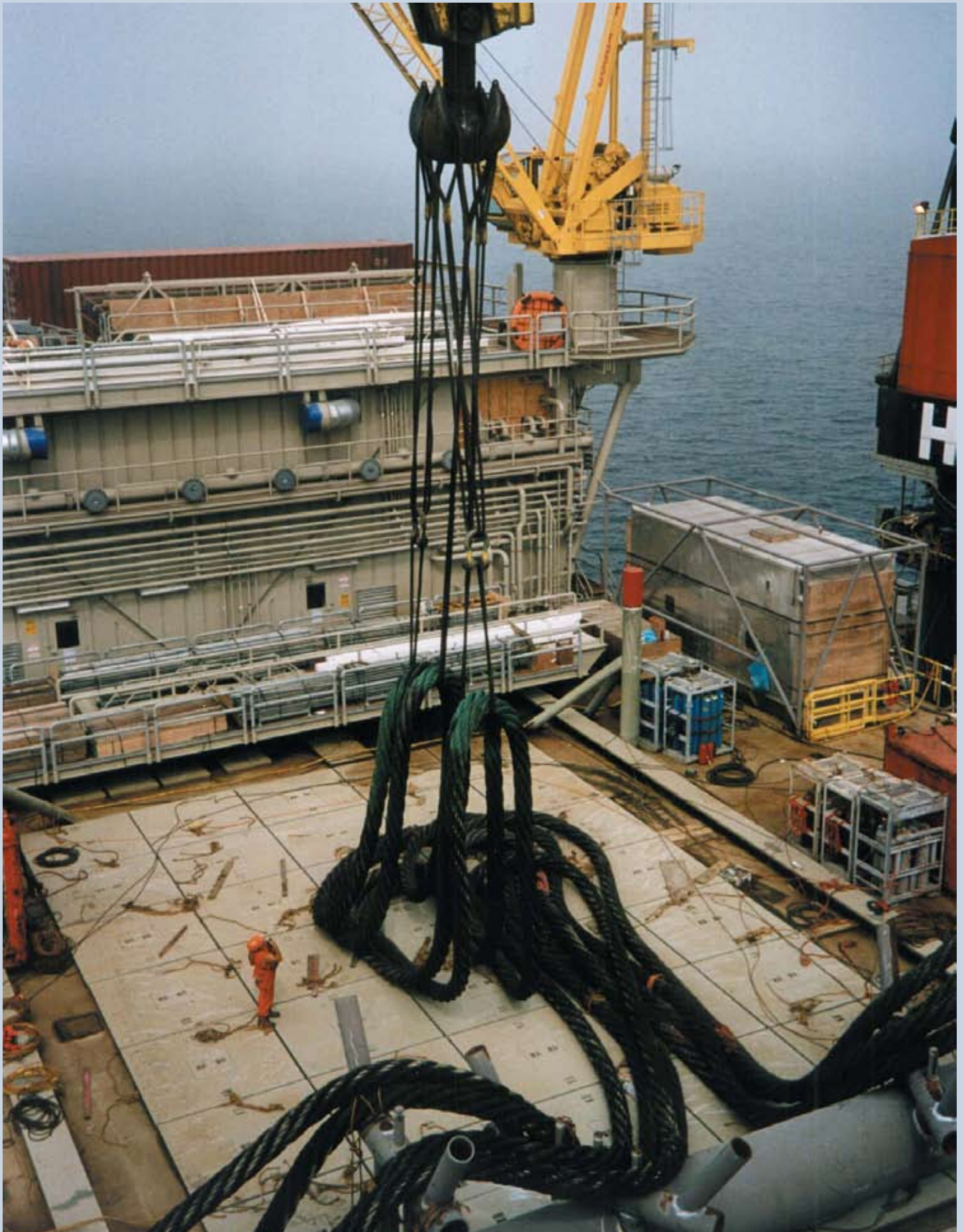
Heavy grommet slings as used on a drilling rig.
